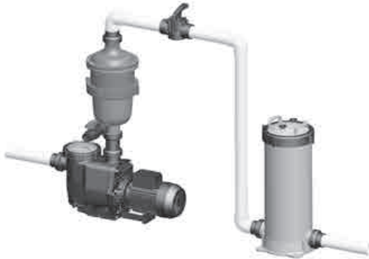
Installation with 2 way shut off valve Cartridge Filter
