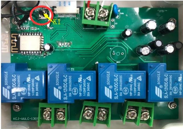
As above photo, the **K1** is the setting key, by pressing it, the lamps can be changed between these 2 modes: Switch on/off control, Controller box control. All lamps' default mode is Switch on/off control mode.
