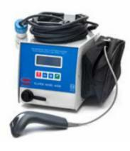
The electrofusion welding unit model Euro MIDI is a polyvalent unit suitable for the welding of all electrofusion fittings up to diameter d. 400. It allows to operator to work at safety voltage lower than 50 Volt, is manufactured according to UNI 10566 and ISO 12176-2 standards, as well as provided with CE mark.
