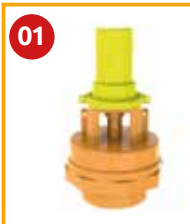
01 Vacuum Relief Valve 1 1/2 Code 5100200012 Setting range: -0,3 bar / -0,8 bar Working temperature: -20°C / +90°C Thread: G 1 1/2 Weight: 0,65 kg
