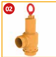
Overpressure Safety Valve - 1 1/4 Code 5100200009 Setting range: +0,3 bar / +1,5 bar Working temperature: -20°C / +90°C Thread: G 1 1/4 Weight: 0,94 kg
