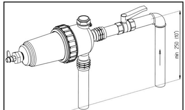
Fig. 2: 90° Angle installation
