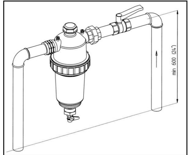
Fig. 1: In-Line installation
