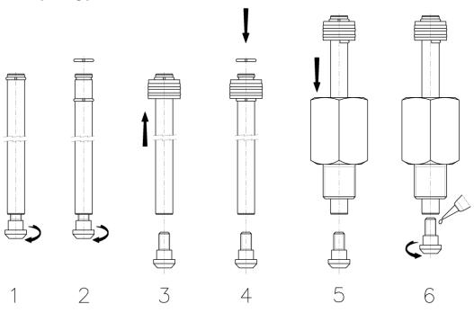
The stem of the cylinders items 0500 - 0510 - 0550 - 0551 is made by two pieces (stem + terminal) and, as a spare part, it is supplied with a pre-assembled stop ring to facilitate the replacing procedure.
