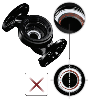
Incorrectly centred sealing system
