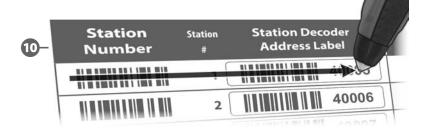
The Successful Scan screen appears and the station # and Decoder # fields will be updated with the scanned barcode data (the screen will always display the most recently scanned data).
