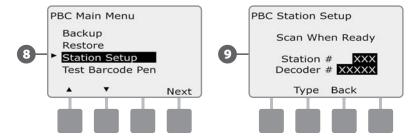
On the Programming Guide, scan a station Number barcode and corresponding station Decoder Address Label in sequence. You'll hear audible beep(s) to confirm when scans are successful.
