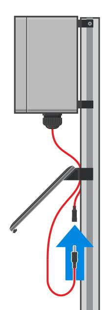
Insert the solar panel's red wire into the slot.
