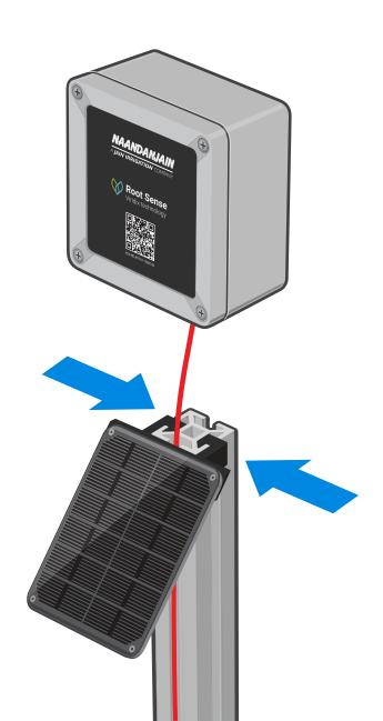
3 Slide the data logger and solar panel down the pole.
