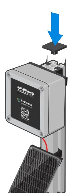
Screw the stopper screws in gently to lock the data logger and solar panel in place.
