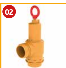
Overpressure Safety Valve 1 1/2 Code 5100200010 Setting range: +0,3 bar / +1,5 bar Working temperature: -20°C / +90°C Thread: G 1 1/2 Weight: 1,02 kg
