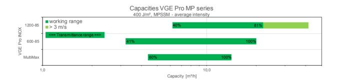
An UV-C dose of  $400 \text{ J/m}^2$  equals  $40 \text{ mJ/cm}^2$  and the transmittance of the water is measured with UV-C light (254 nm) through 10 mm of water.
