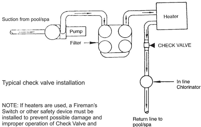
NOTE: If heaters are used, a Fireman's Switch or other safety device must be installed to prevent possible damage and improper operation of Check Valve and other equipment subject to heat damage.
