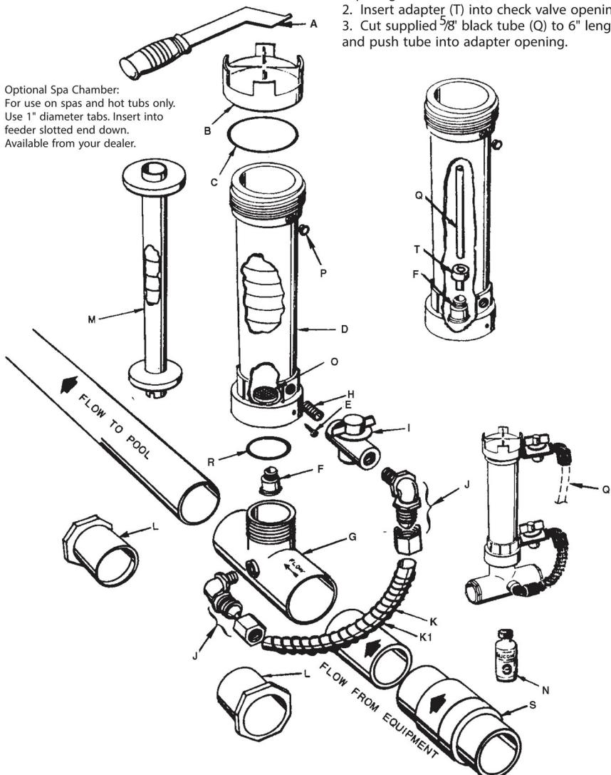
YOU MAY SUBSTITUTE BROMINE TABLETS OR STICKS FOR TRICHLOR IN THIS FEEDER. DO NOT MIX.
