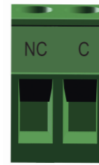
Relay output in the control box
