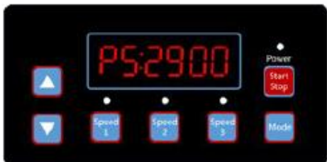
(Diagram 6.22, Selv Priming Hastighed, standard 2900rpm)
