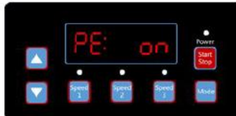
(Diagram 6.23, Selv Priming Aktiver/Deaktiver, Standard Til)
