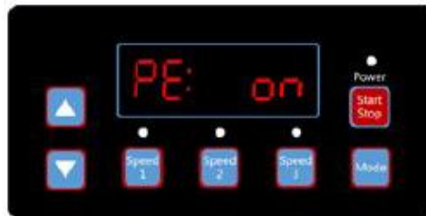
(Diagram 6.21, Selv Priming Tid, standard 2 minutter)
