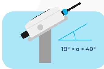
2. Place the device facing the sun. In Spain, for example, to the south at an angle of 30°.
