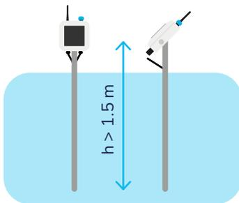
1. Screw the device firmly onto a support, 1.5 meters above the ground.
