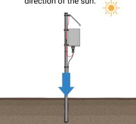
Place the sensors in the soil in the desired depths and cover with soil. Avoid gaps between the sensors and the soil. Wet the area around the sensors.
