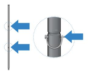
Connect the data logger and solar panel to the pole.
