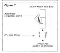
7. Insert the end of the hose through the skimmer opening and connect the hose directly onto the automatic regulator valve.
