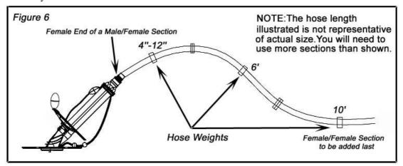
The body is connecting with hose; please refer to the right picture. Only model# D needs to use an adapter to connect the hose.
