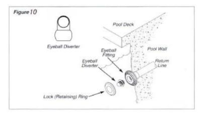
Position the diverter opening to redirect the return line water flow so it does not interfere with the cleaner's movement. Try different positions to see which works best in your pool:
