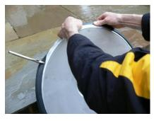
4. Hold on side and push/pull in opposite direction the inlet and outlets to rotate the two filter haves in to the correct positions to align with your installation pipe work
